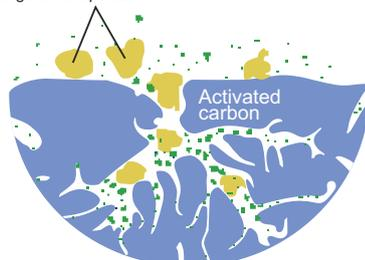
Raw water wraps the block from the outside towards the core. Chlorine and its derivatives are retained on the surface, and the purified water flows into the inside of the cartridge.
